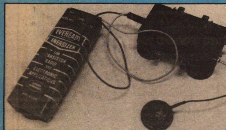
CMSS found this transmitter attached to a car by its large magnets. The huge battery could power it for about five days.
